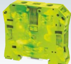
CGT 50/70N 70 x 77 x 20.5 mm 10.0 - 70.0 mm 2 192 A, 1000 V, 3.0 Nm
