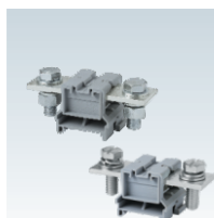
CBB150 / CBB150LS 47.3 x 110 x 48 mm 16.0 - 150.0 mm 2 309 A, 1000 V, 14.0 Nm
