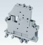
CF4SP / CF4SPL# 70.0 x 58.5 x 6 mm 0.2 - 4.0 mm 2 , 6.3 A, 1000 V, 0.5 Nm, Fusível Ø5x20 mm
