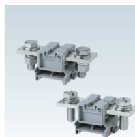
CBB185 / CBB185LS 47.3 x 110 x 48 mm 16.0 - 185.0 mm 2 353 A, 1000 V, 14.0 Nm
