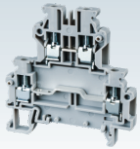
ODL2.5A 61 x 59 x 5 mm 0.2 - 2.5 mm 2 24 A, 800 V, 0.4 Nm
