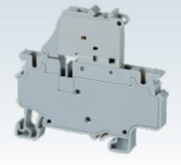
CXF4 / CXF4L 61.5 x 65.4 x 6 mm 0.2 - 4.0 mm 2 10 A, 1000 V
