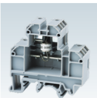
CDL4U(E)LA 55.7 x 55.5 x 18 mm 0.25 - 4.0 mm 2 , 10A, 0.5Nm 75 - 1000 VCC/20 KA (8/20 μs)
