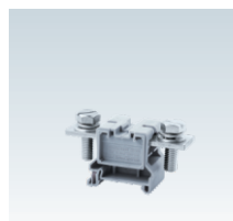
CBB95LS 47.3 x 92 x 38 mm 16.0 - 95.0 mm 2 232 A, 1000 V, 10.0 Nm
